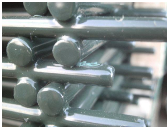
Paint damage by shifting
