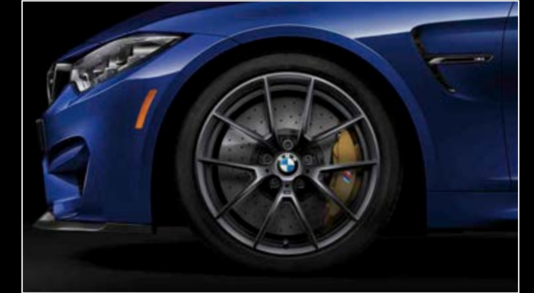
19" / 20" M Double-spoke forged wheels, style 437M 19 x 9.0 front, 20 x 10 rear; and 255/35 front, 285/30 rear performance 1,2 non run-flat 3 tires
