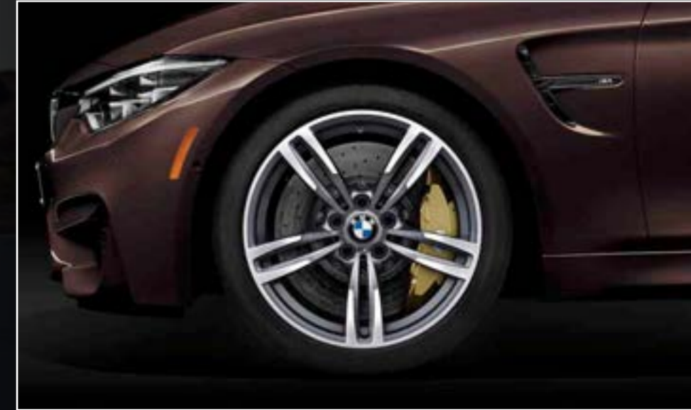
19" M Double-spoke forged wheels, style 437M 19 x 9.0 front, 19 x 10 rear; and 255/35 front, 275/35 rear performance 1,2 non run-flat 3 tires
